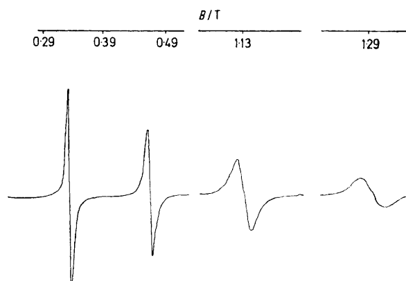
FIGURE 3 X-Band spectrum of a single crystal of \text{La}[\text{N}(\text{SiMe}_3)_2]_3 doped with \text{Gd}^{3+} aligned with the magnetic field parallel to the trigonal axis
